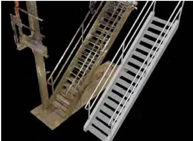
Comparison between a scanned point cloud on the left and a resulting 3D model on the right
