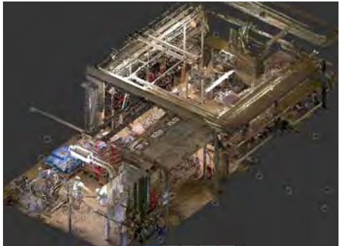
Point cloud of a complete building including plant engineering
