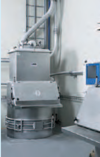
Feeding hopper for discharging bags into the closed system
