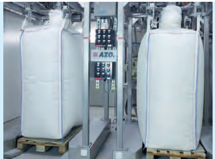
Automatic big-bag feeding with precise accuracy
