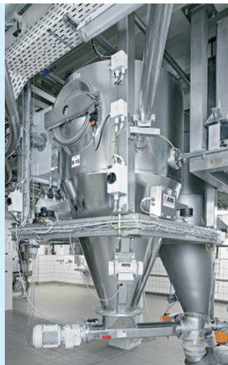
Conveying scales for feeding a kneading machine with sugar
