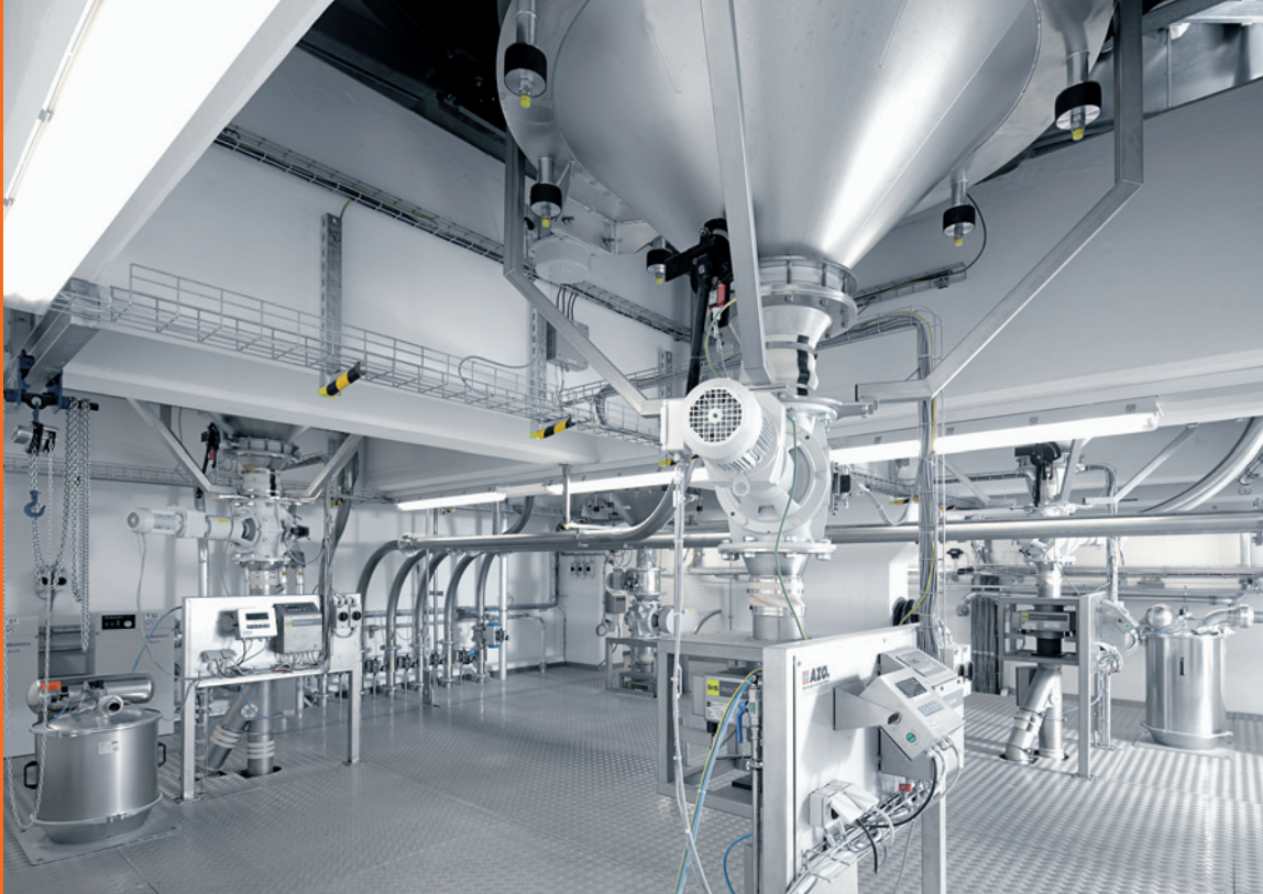
Product discharge from silos with metal separation
