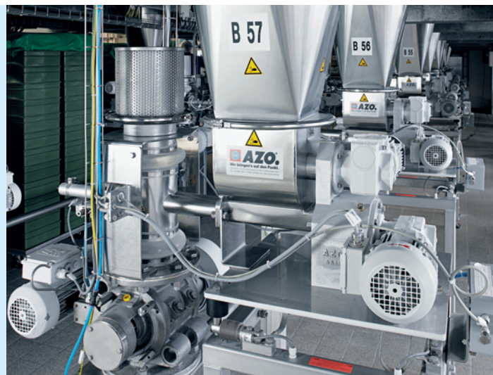
AZODOS® equipment for precise weighing of small quantities
