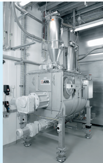
Powdered sugar hopper with agitator
