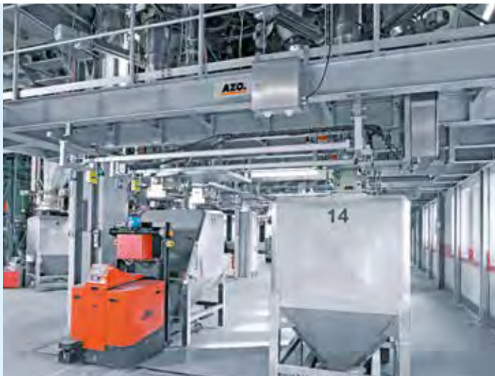
According to the recipes the AGVs move to the scales hanging in the platform
