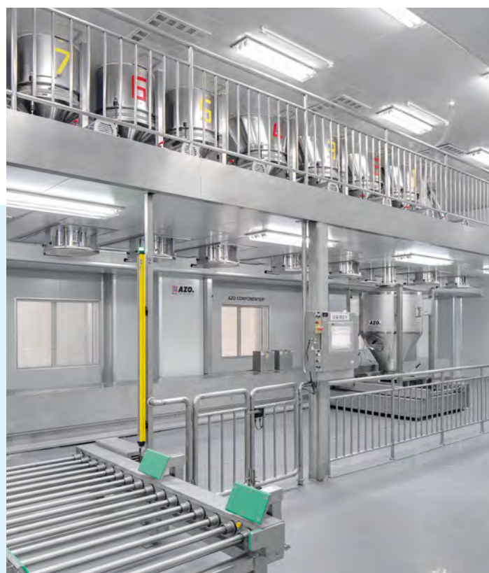
Automatic weighing using the AZO COMPONENTER®
