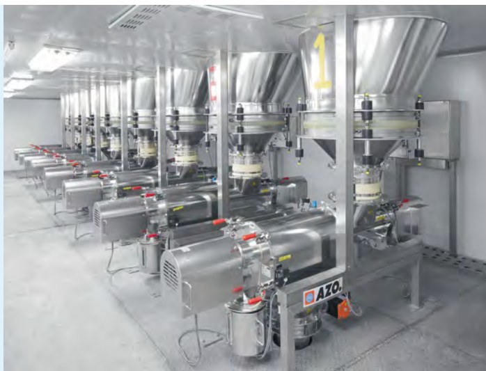
Cyclone screeners below the feeding hoppers for control screening
