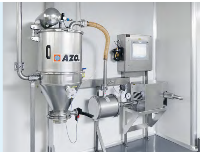
Central extraction of dust from the docking devices with upstream secondary filter
