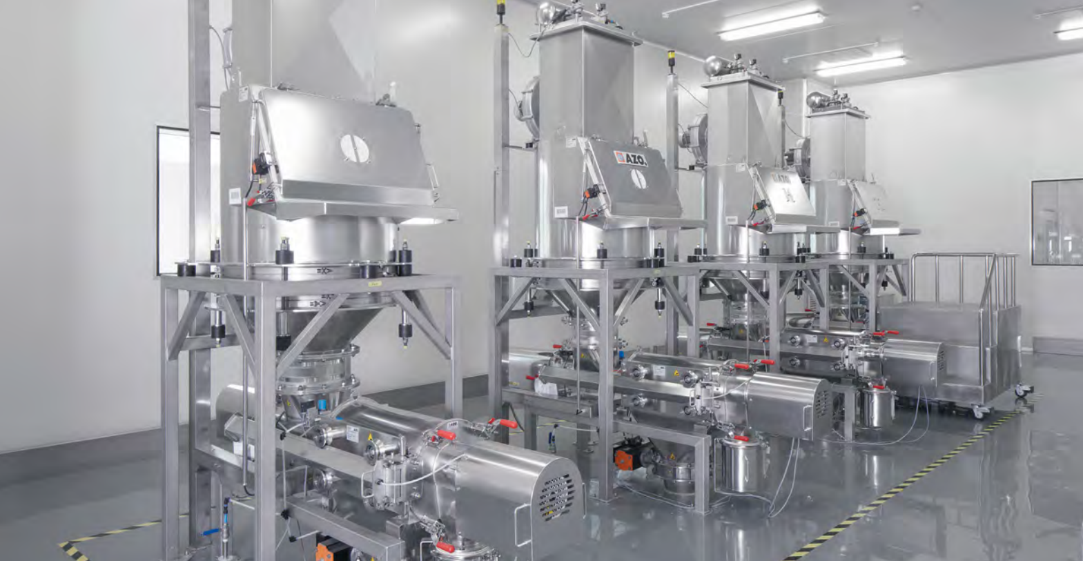
Feeding hopper with cyclone screeners ensure that bagged goods are fed reliably with little generation of dust
