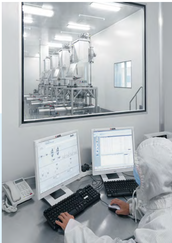
Control room with process control and visualisation system
