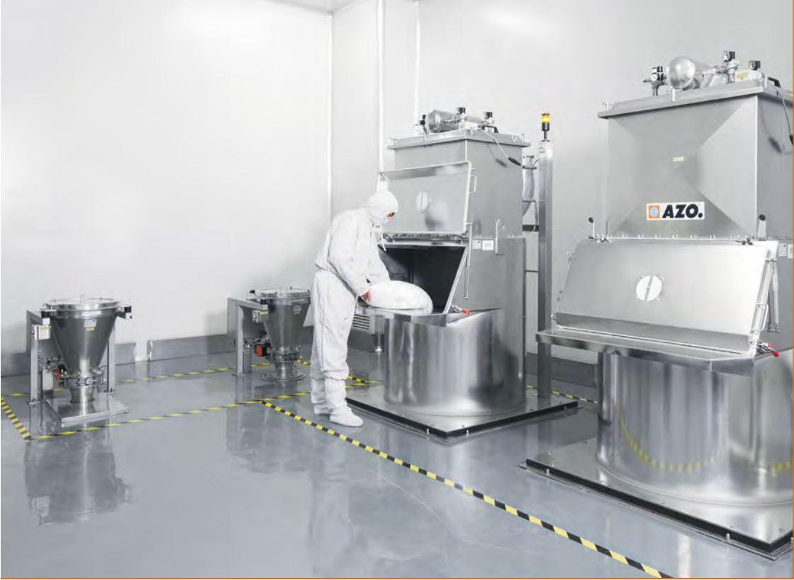
Feeding hopper with integrated filters ensures that there is little generation of dust while feeding bagged goods
