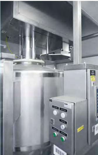
Docking device with trickle guard slider
