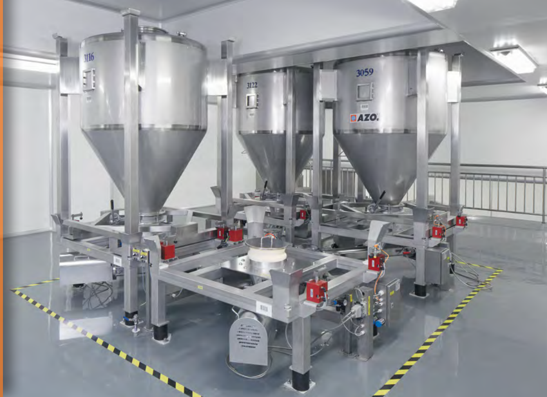
BATCHTAINER® discharge bases with patented docking collars and frequency controlled dosing screw
