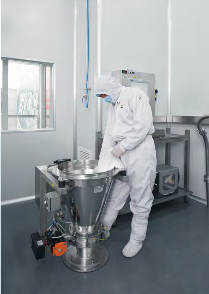
Feeding funnel for the small quantities that are pre-weighed at the ManDos
