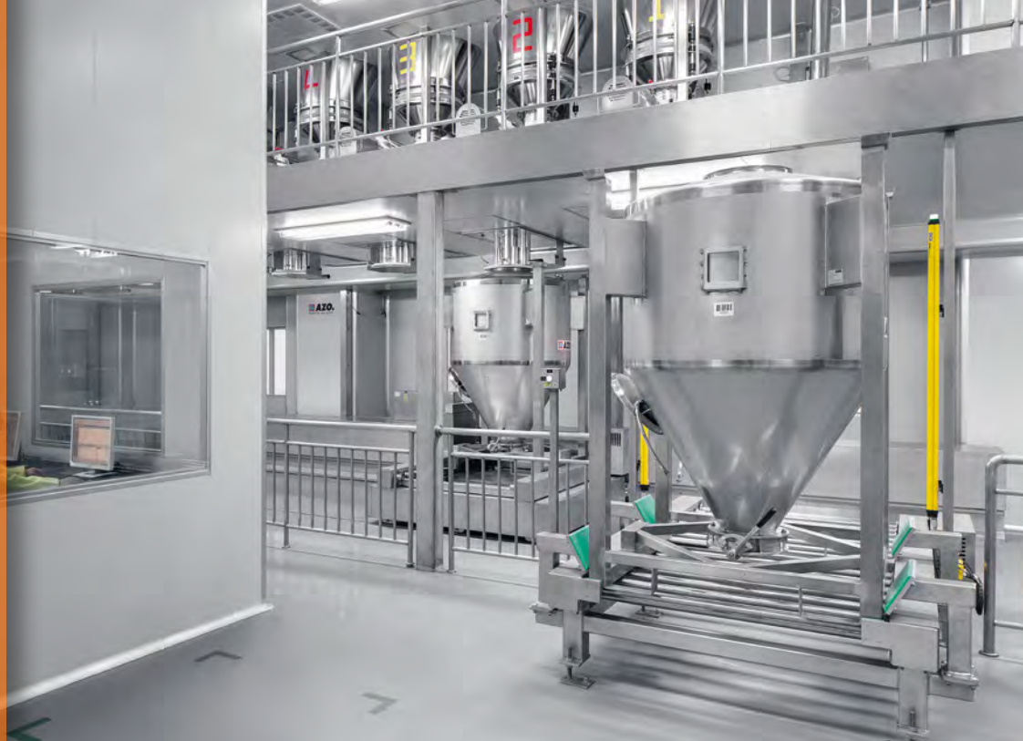
Removal of the filled BATCHTAINER® from the AZO COMPONENTER®
