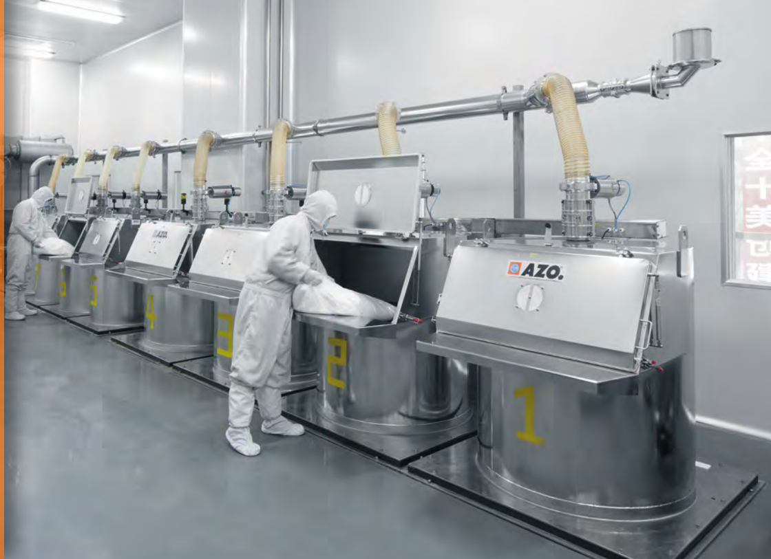
Feeding hopper for feeding raw materials with little generation of dust on the top level of the AZO COMPONENTER®
