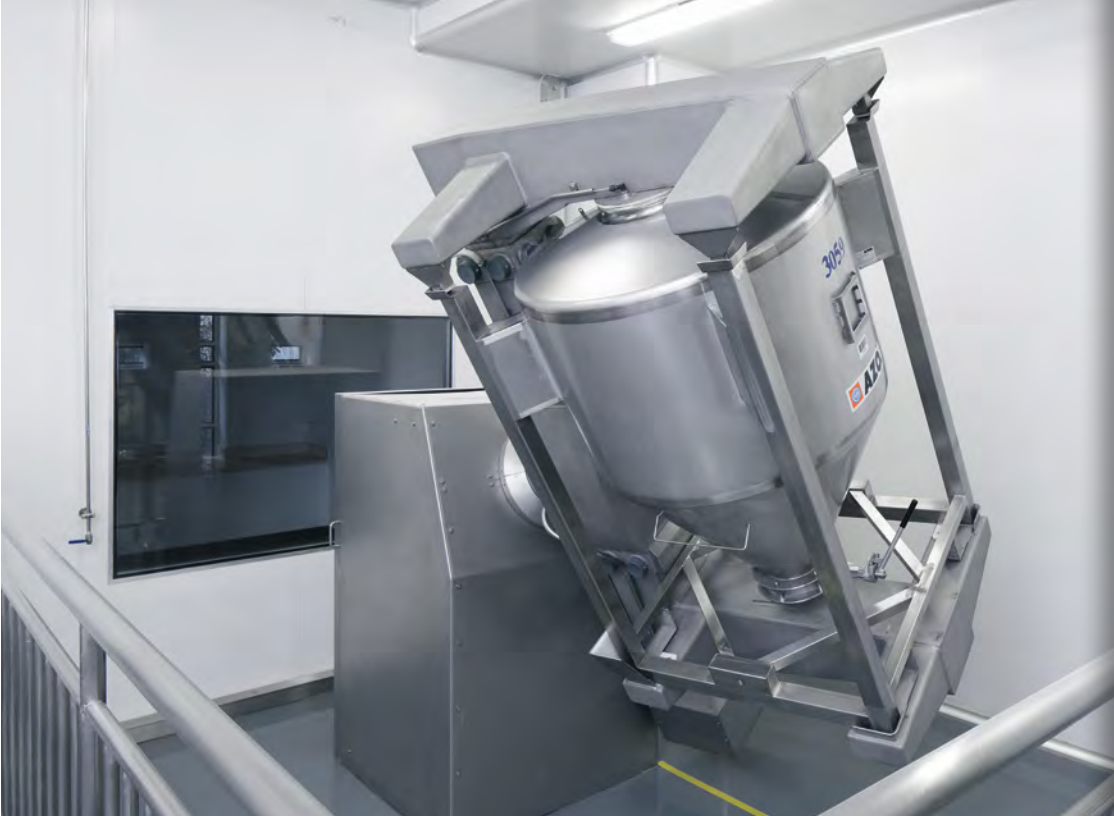
Container mixer for producing homogeneous ready mixes
