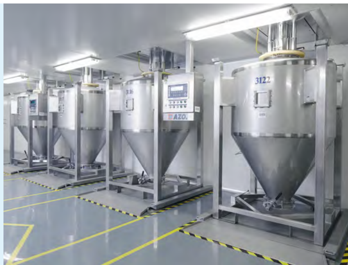
Weighing of raw materials into BATCHTAINERS® on floor scales
