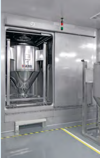
Hygienic wet cleaning of BATCHTAINERS® in the container washing line
