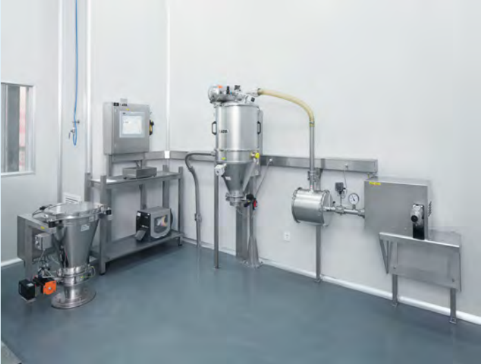
Left: ManDos with feeding funnel Right: central extraction of dust from the docking devices with upstream secondary filter
