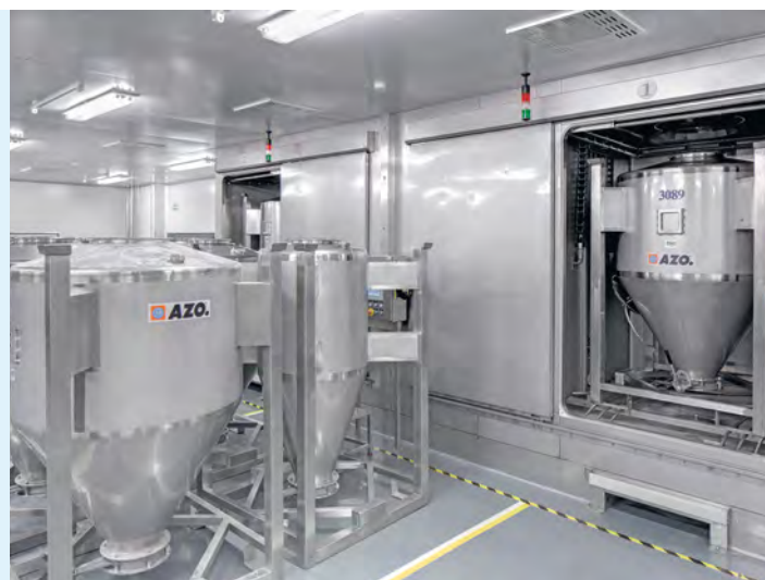
Container washing system for rigorous wet cleaning of used containers
