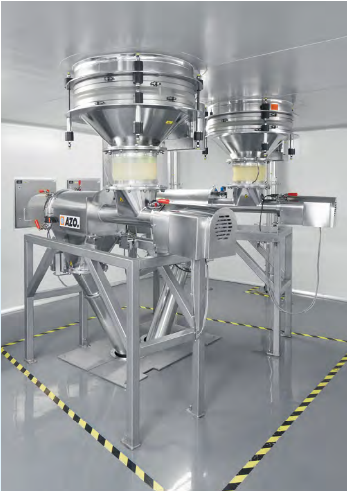
Cyclone screener for control screening and dosing
