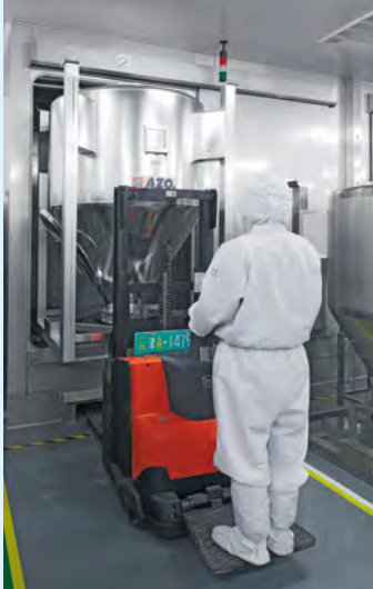
Hygienic wet cleaning of BATCHTAINERS® in the container washing line
