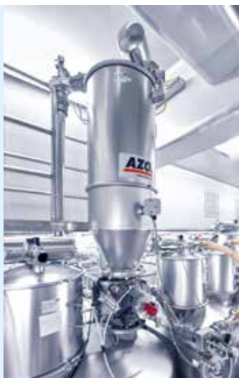
Continuous conveying of the bulk component A into the buffer hopper
