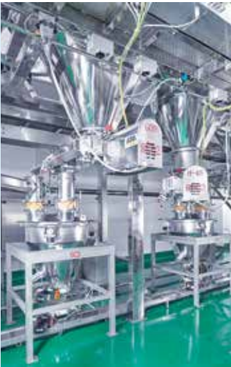
Accurate weighing of minor quantities in hopper scales
