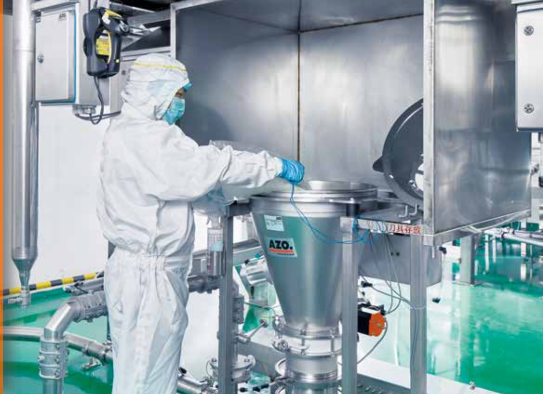
The machine operator fills the pre-weighed and labelled batch into the feeding hopper
