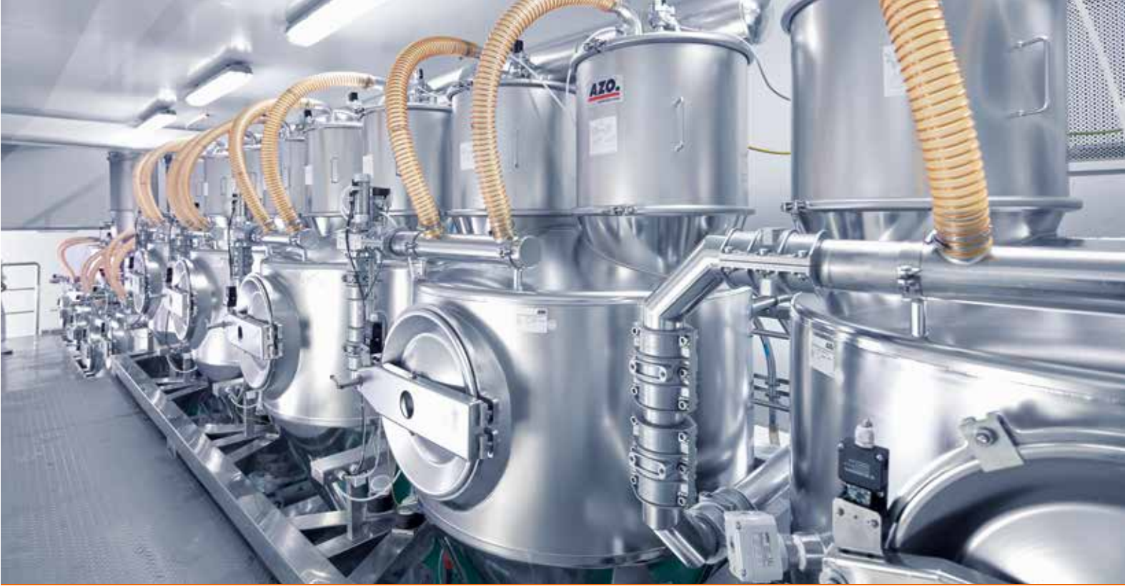
Closed pneumatic conveying systems ensure production with a minimum of dust
