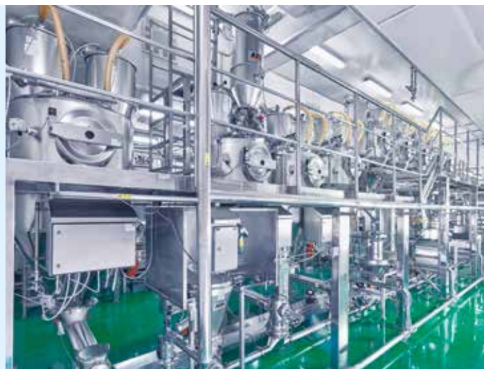
The components are metered from the buffer hoppers into the vacuum weighing system
