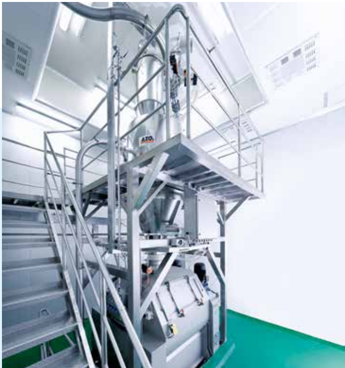
Reliable feeding of the mixer via a vacuum weighing system
