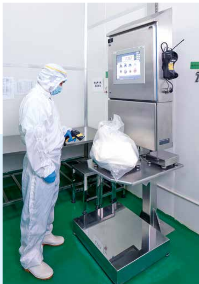
ManDos computer-aided manual weighing system for precise weighing of micro quantities
