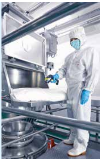
Product feeding with monitoring of barcodes
