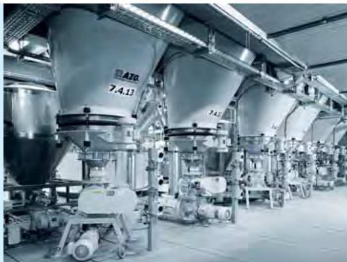
Day silos, equipped with vibration bottoms and rotary valves, some with cyclone screeners on their output ends
