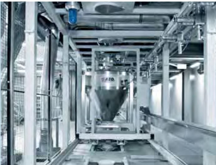
The hopper of the mobile scale can be replaced when there is a product change
