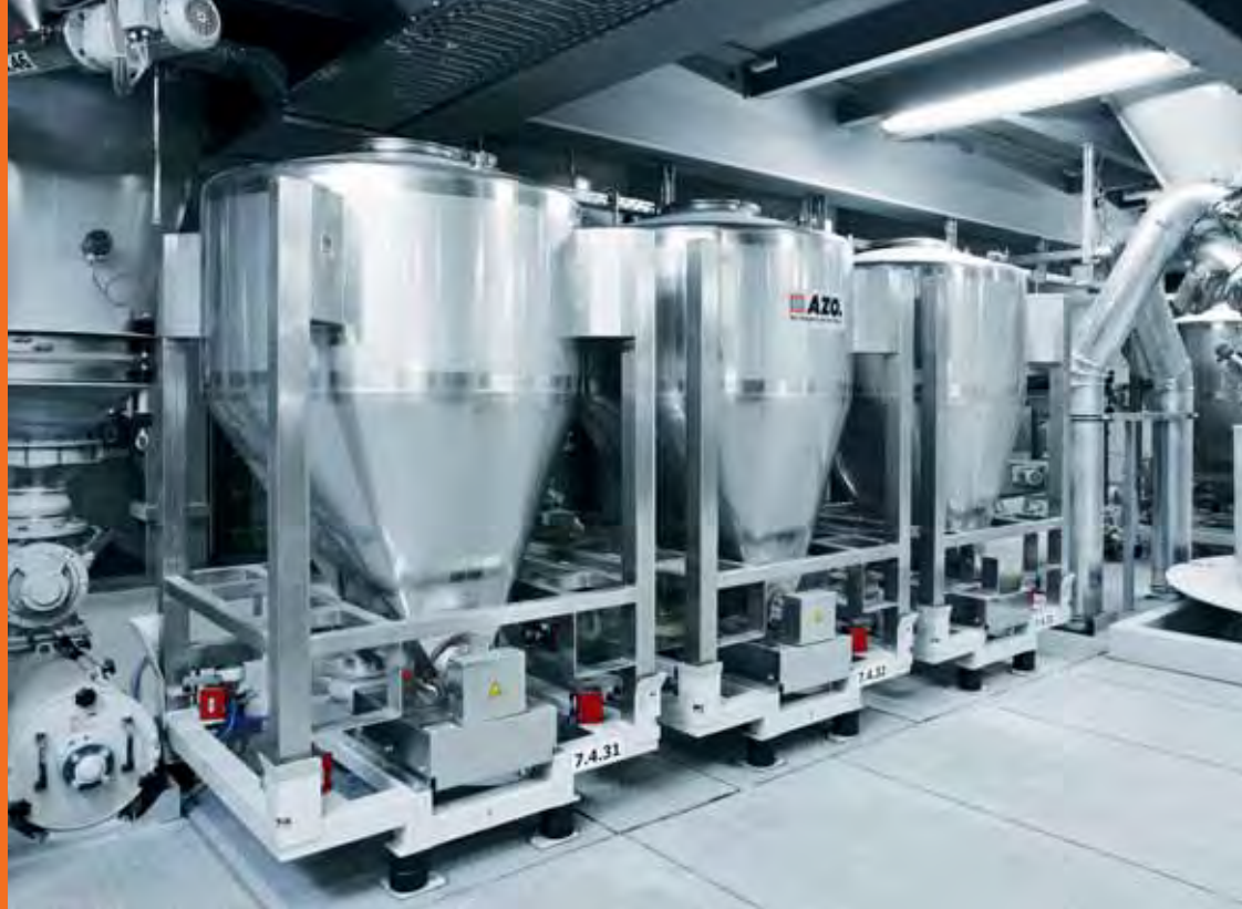
AZO DOSITAINER® with integrated dosing screw as flexible product additions in the AZO COMPONENTER®
