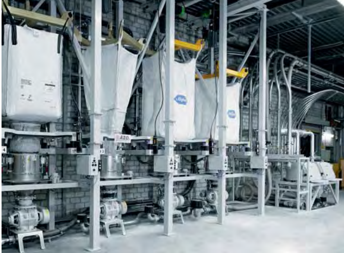
Big bag discharge stations for feeding the product into the closed system without dust
