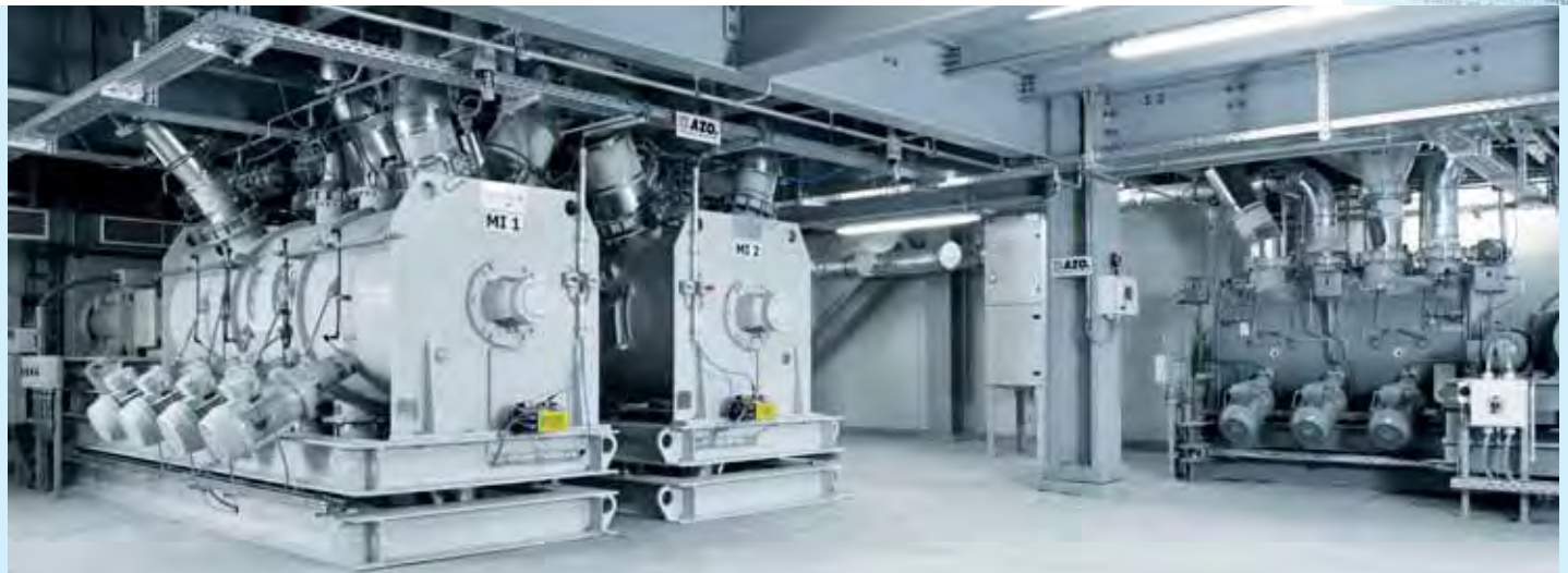
Two horizontal shaft mixers for manufacturing standard products, right: a mixer for premixes and special products
