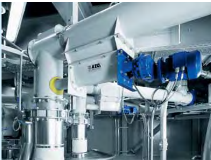
Dosing screw followed by ultra-precise dosing
