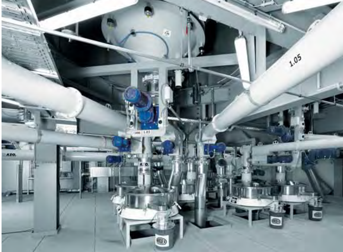
Safe product outfeed via vibration bottoms and dosing screws with subsequent control screening
