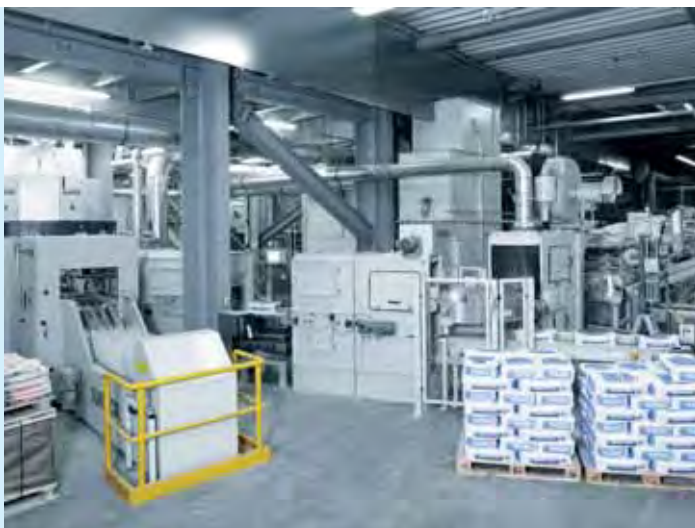
Automatic bagging and palletising machine
