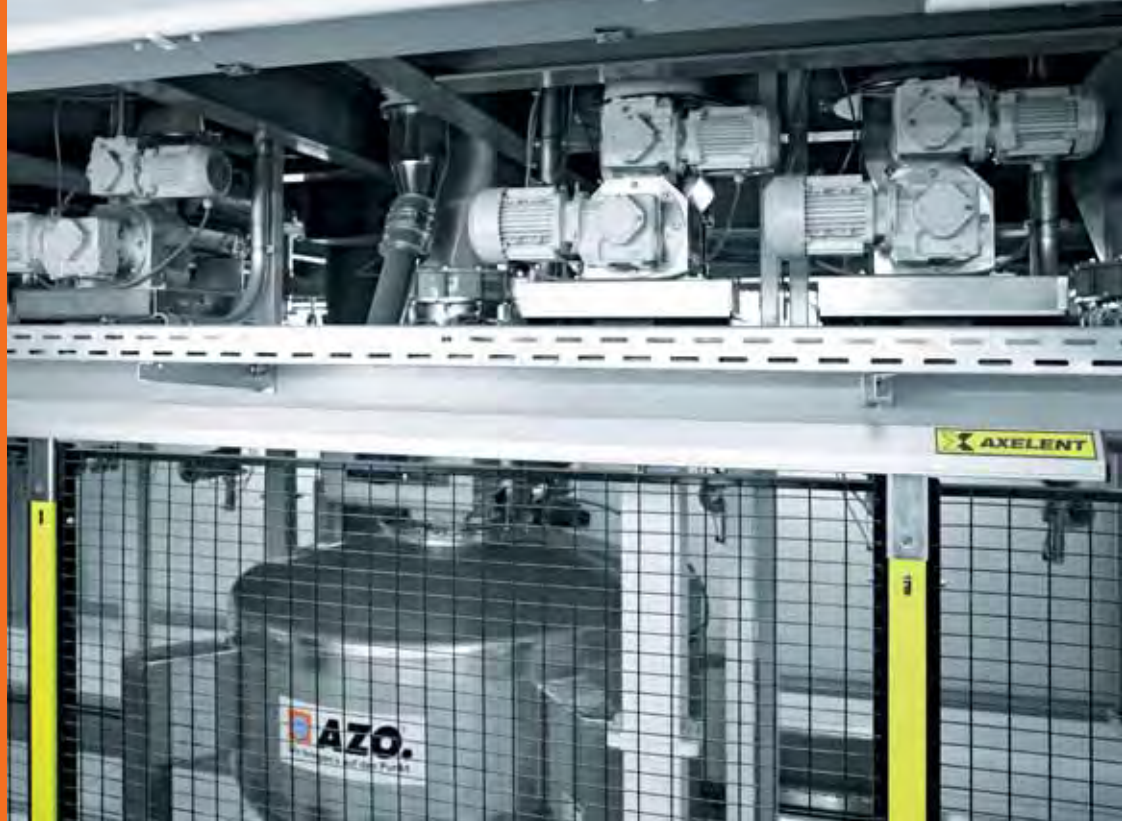
AZODOS® units allows to weigh accurately the minor components into the mobile scale
