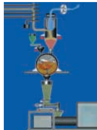
Feeding of minor quantities directly into the MIXOMAT
