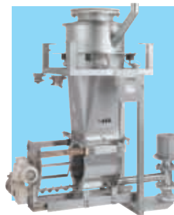
Mixer fully withdrawn and dosing screw partially withdrawn
