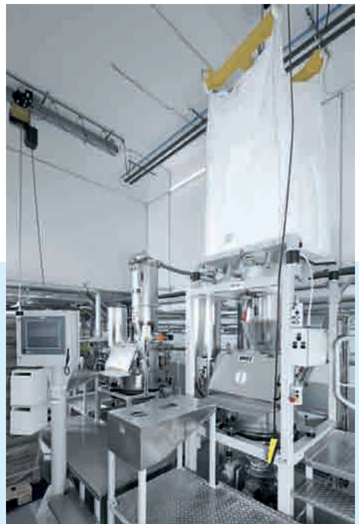
Big bag discharge station with integrated feeding hopper and central aspiration system
