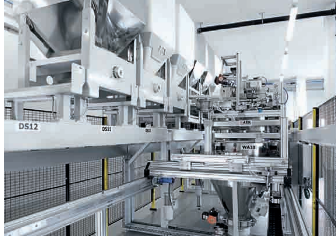
Mobile scales of the DOSINENTER® with docking systems for DosiBoxes® and DOSITAINERS®
