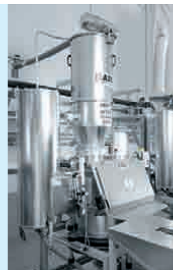
Feeding hopper with empty bag compactor and additional receiver for pneumatic filling
