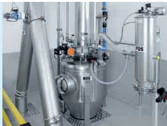
AZO®MULTIAIR dense-phase conveying system for the gentle conveying of the finished granulate
