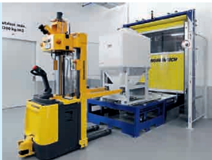
Automatically guided fork truck for the automatic handling of raw material containers
