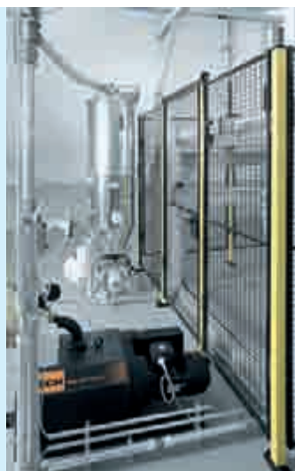
Vacuum conveying system for the feeding of the compactor roller
