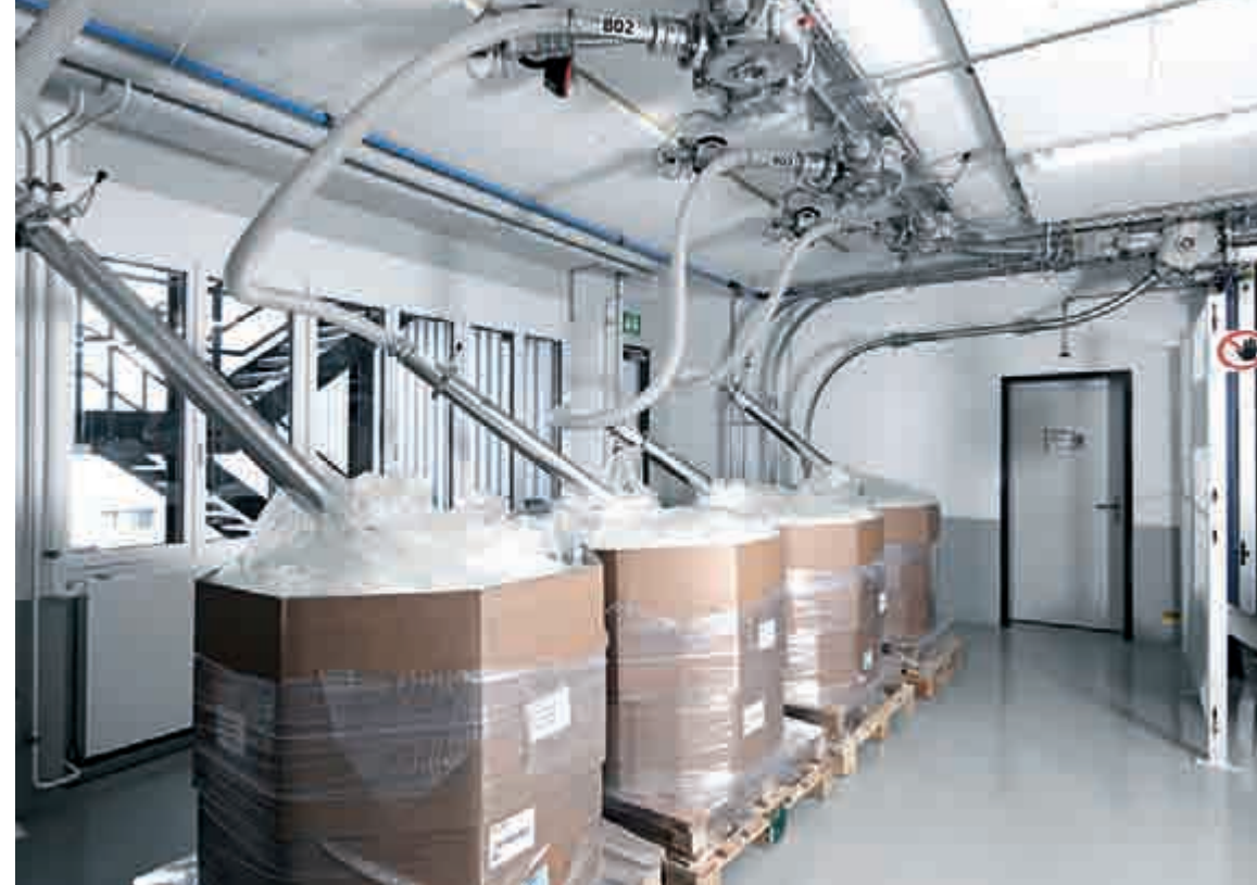
Clean feeding of medium-sized components from octabins by means of vacuum conveying systems
