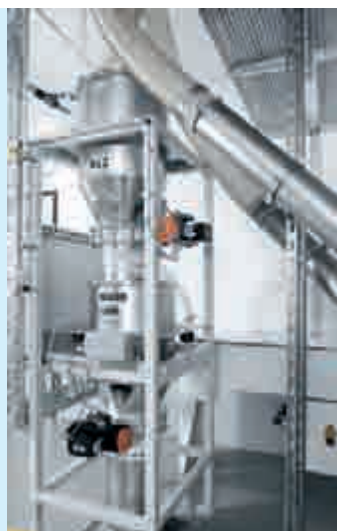
Throughput recording and sampling of the finished compound
