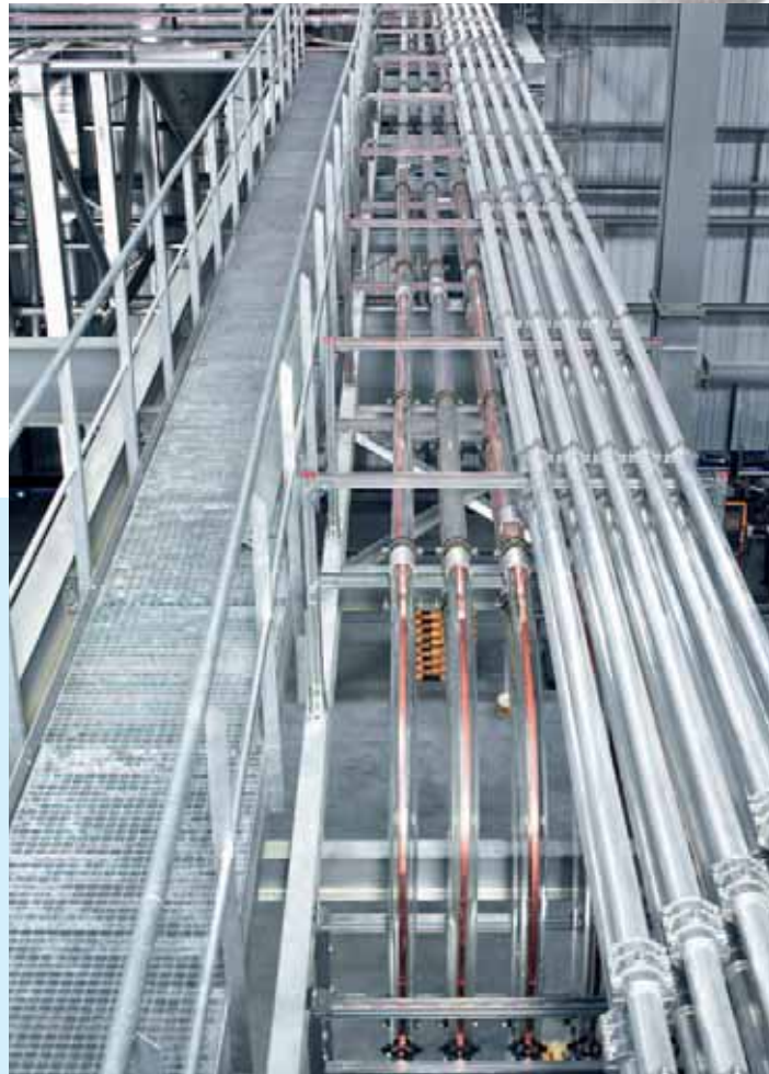
Conveying tubes made from glass with copper grounding reduce wear from abrasive products
