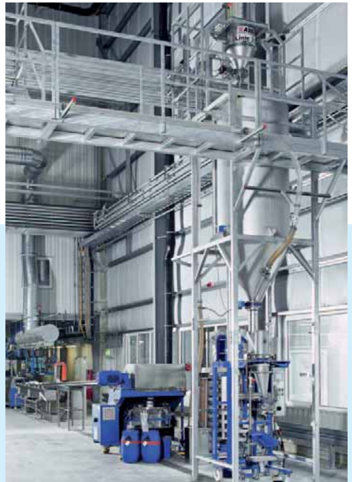
Extruder screw with pelletiser, screen and helical cooler as well as a day bin with bagging line
