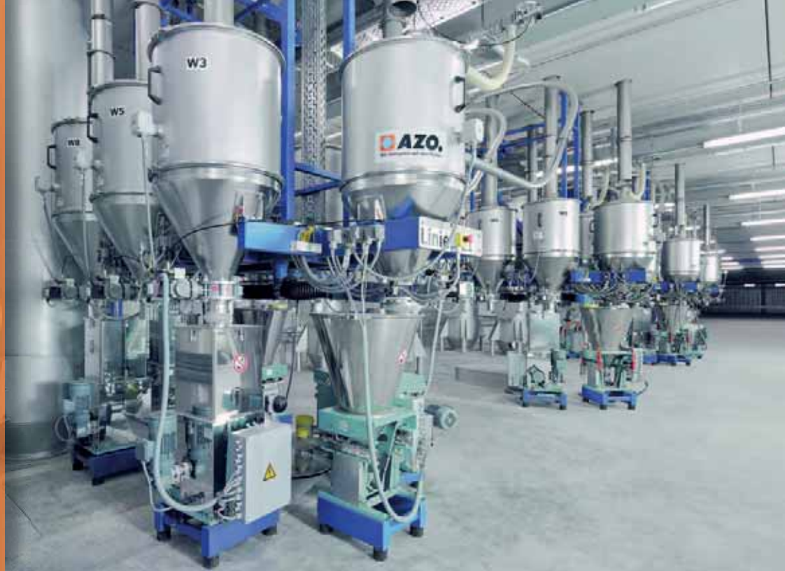
Extruder filling via loss-in-weight feeders
