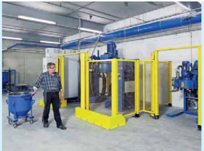
A homogeneous mixture is generated directly in the container using the container mixer.
