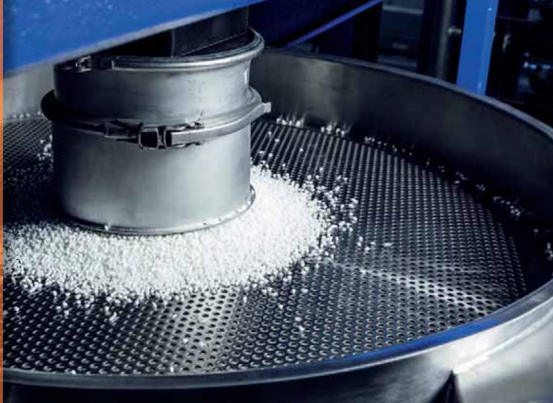
Flat vibrating screen for separating oversize and undersize pellets
