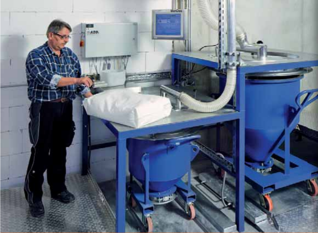
Manual ManDos station for precise weighing to the exact gram and feeding micro quantities
