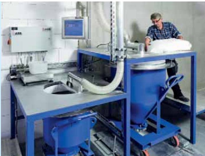
Manual ManDos weighing station for discharge of pre-weighed bags into mixing containers
