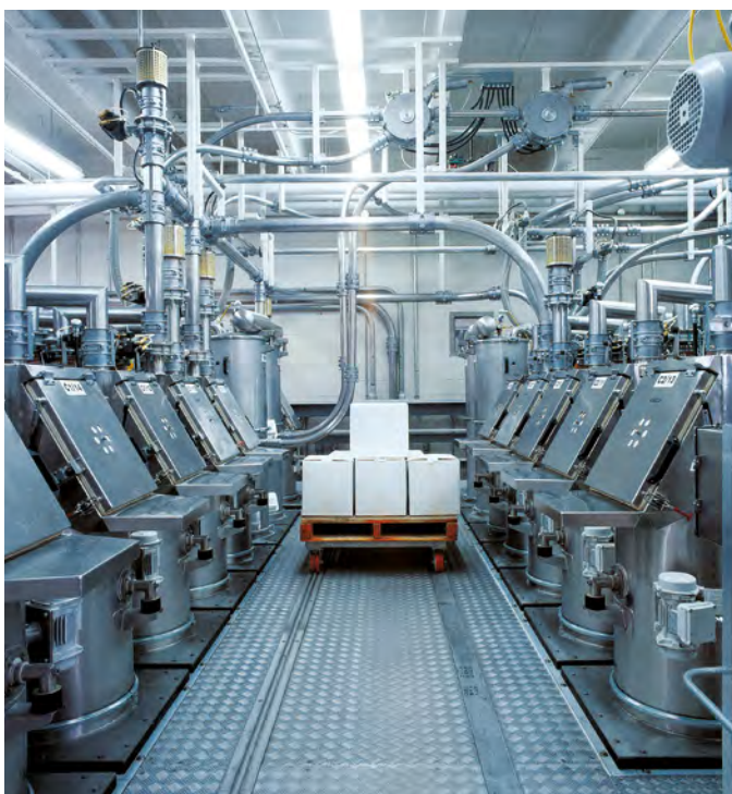
Feeding of the AZO COMPONENTER® via feeding hoppers
