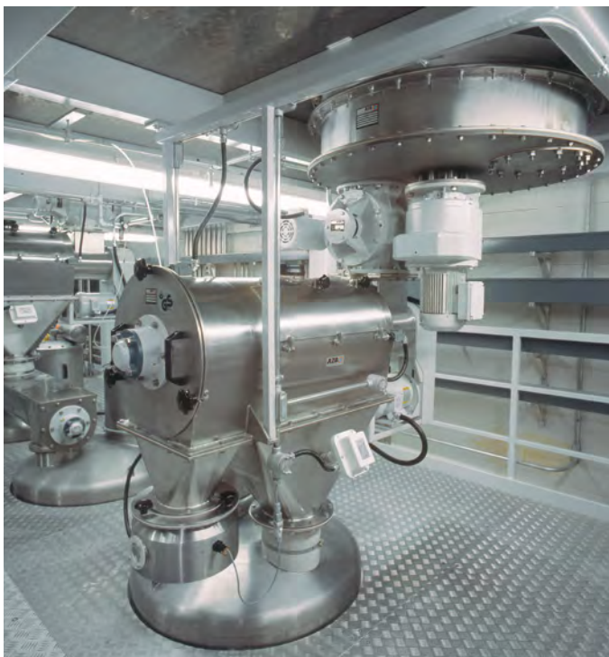
Cyclone screener for safety screening
