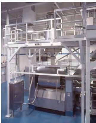
Feeding of kneading machine with vacuum weighing system
