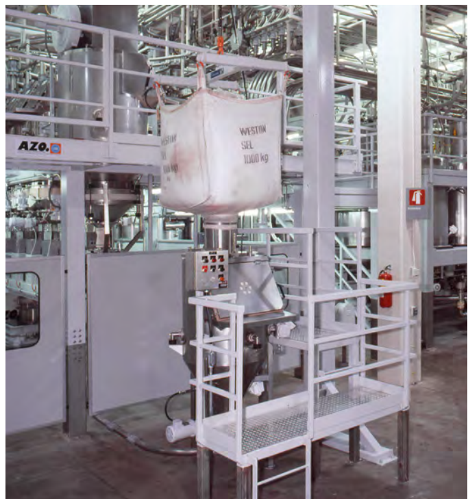
Big bag discharge station and feeding hopper for the feeding of big bags and small sacs
