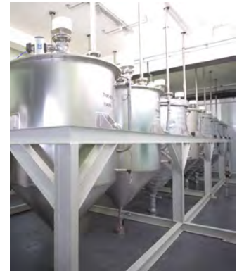
Storage of bulk liquid ingredients in tempered tanks
