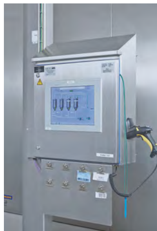
Hygienic design for the operator terminals in the kneading lines
