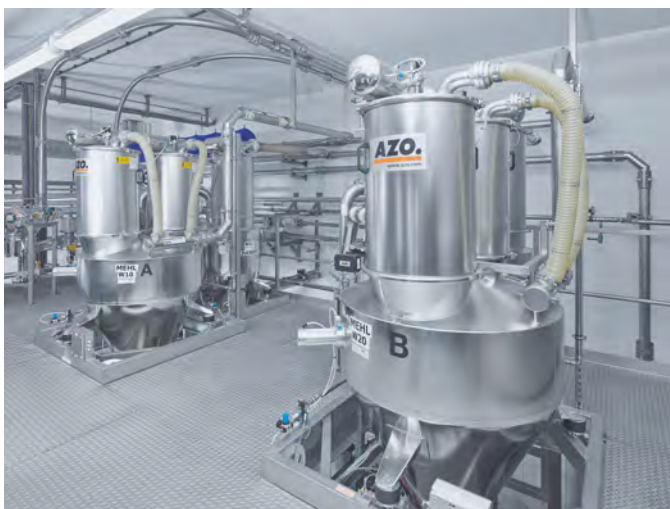
Vacuum weighing systems with conveying scales for flour and sugar
