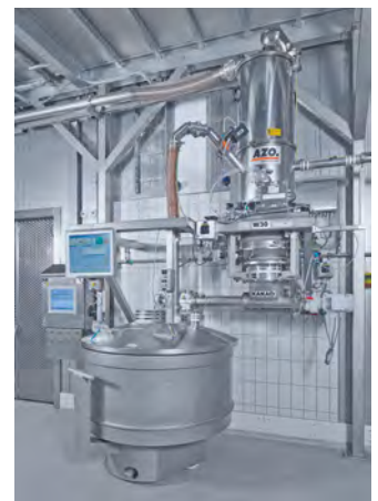
Vacuum weighing system with conveying scales for cocoa
