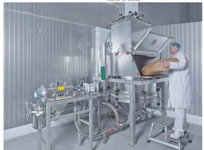
Feeding of cocoa and ingredients with control screening via a separate line
