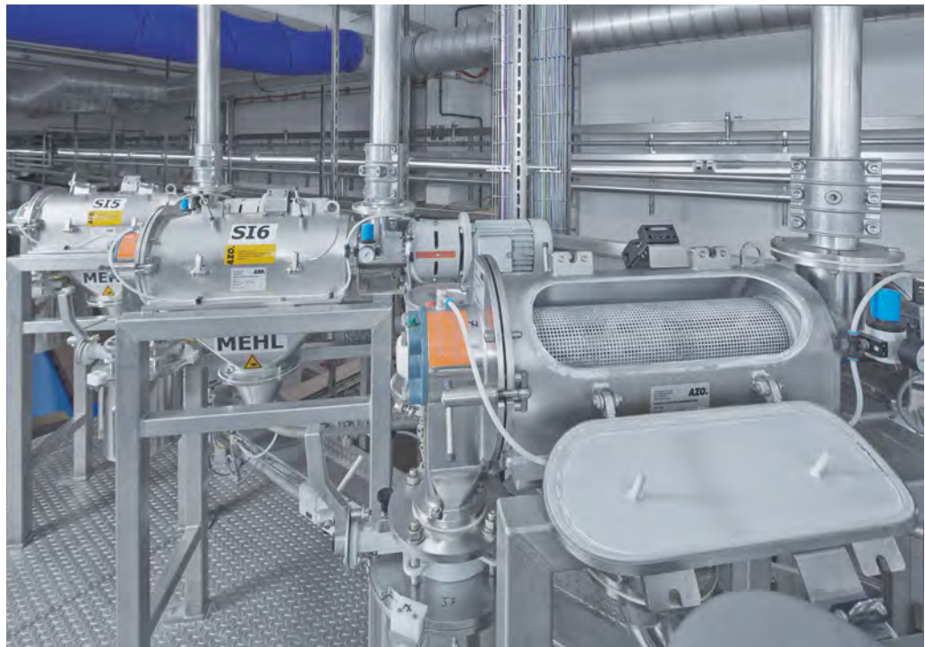
Cyclone screener in the flow for control screening of flour and sugar
