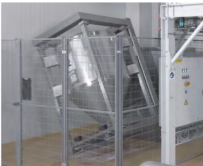
Container mixer for producing homogeneous dry ingredient mixtures
