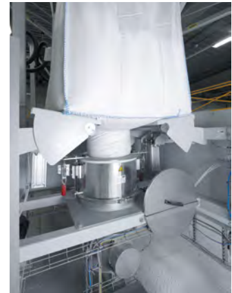
Big bag discharge station with massager device
