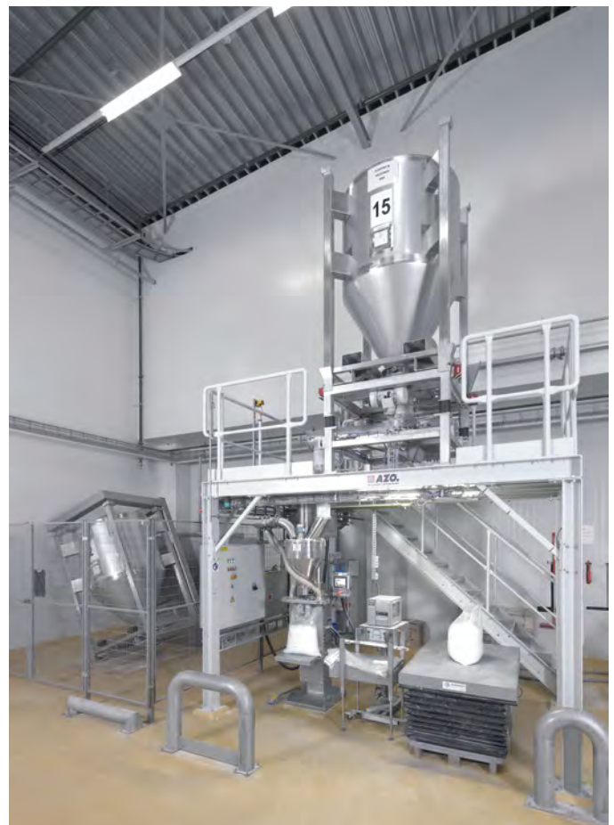
Semi-automatic bagging line for filling the dry mixes into bags and sacks
