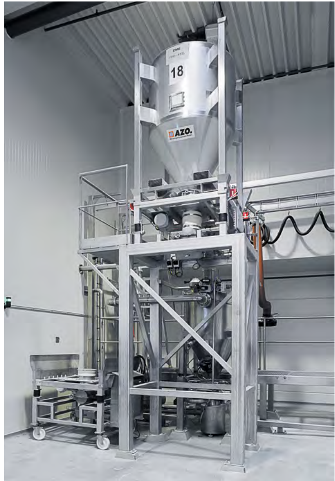
Container station for feeding an inline mixer Left: mobile station for feeding the agitator vessels
