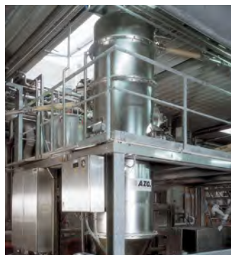
Vacuum-pressure weighing system with CO 2 pressurization
