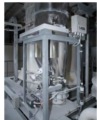
Reception hopper above mixer
