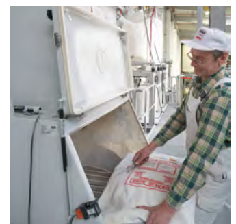
Product feeding from sacks into the closed system
