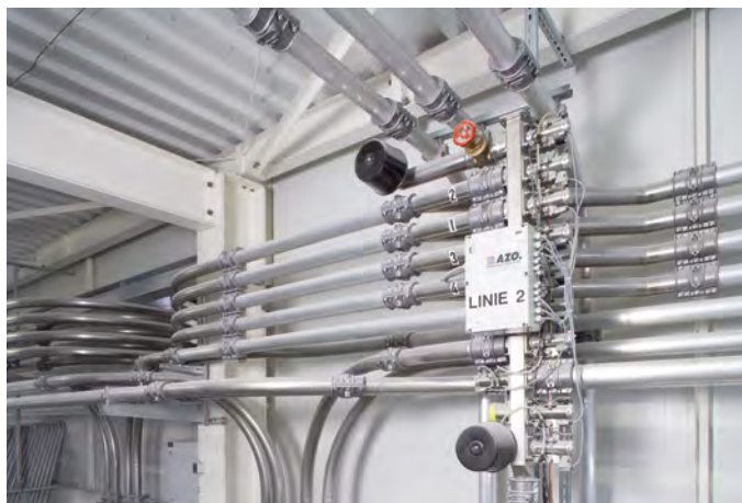
Patented multiport valves transfer the raw materials right to the point
