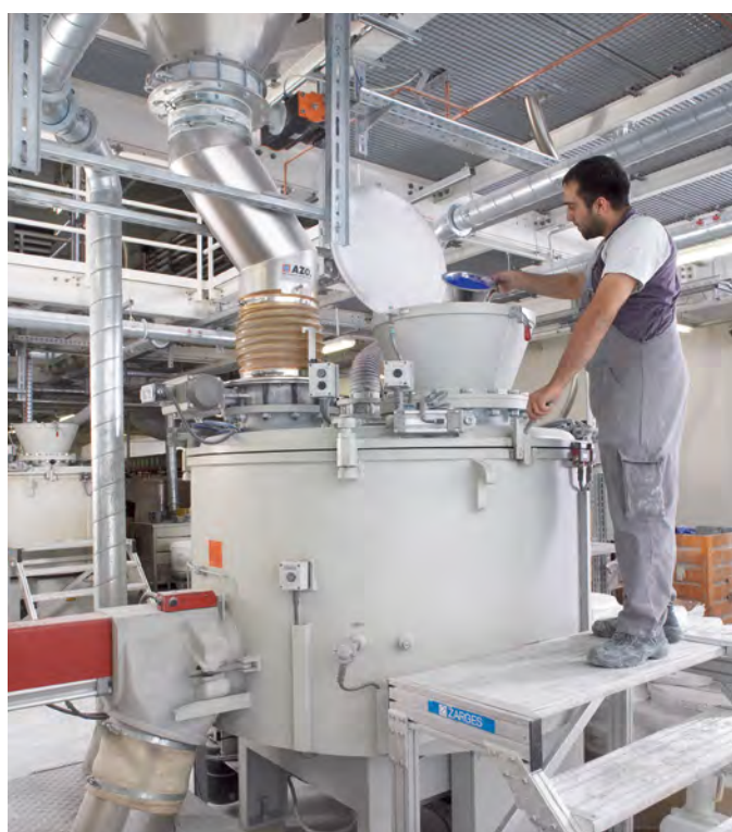
Mixer feeding with feed of the aggregates, dyes, additives
