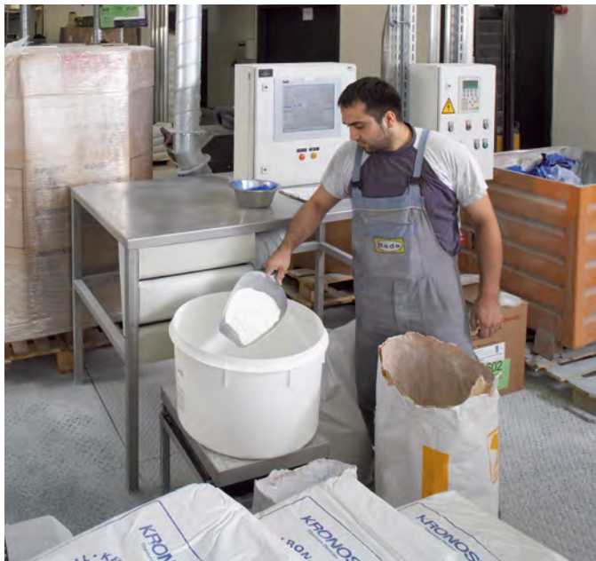
ManDos, operator-guided manual weighing of dyes, additives and aggregates
