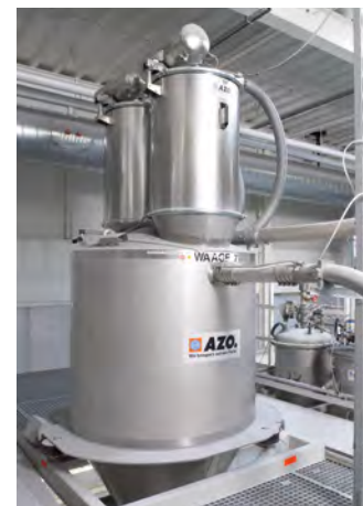
Vacuum weighing systems for major ingredients
