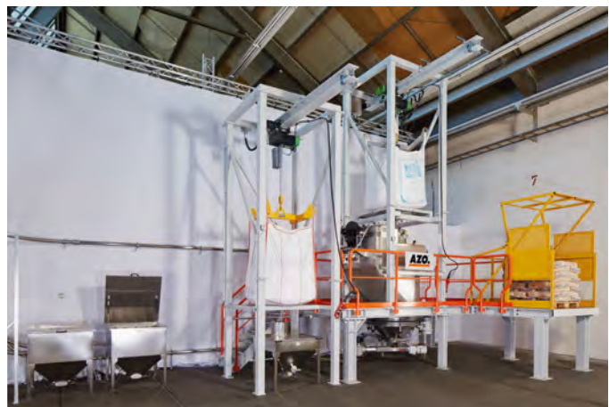
Feeding of raw materials in powder and granulate form
