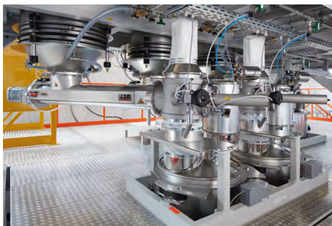
Dosing screws are used to fill the AZODOS® units
