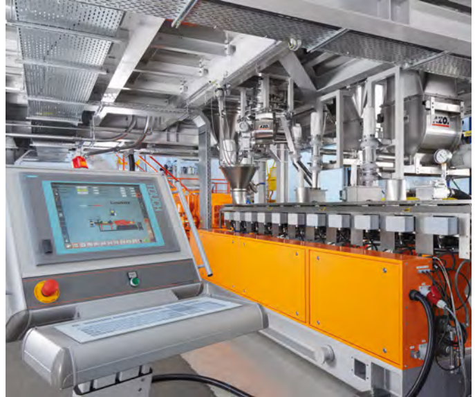
MacromateXX S7 professional from Leistritz for controlling the extrusion process and all downstream units
