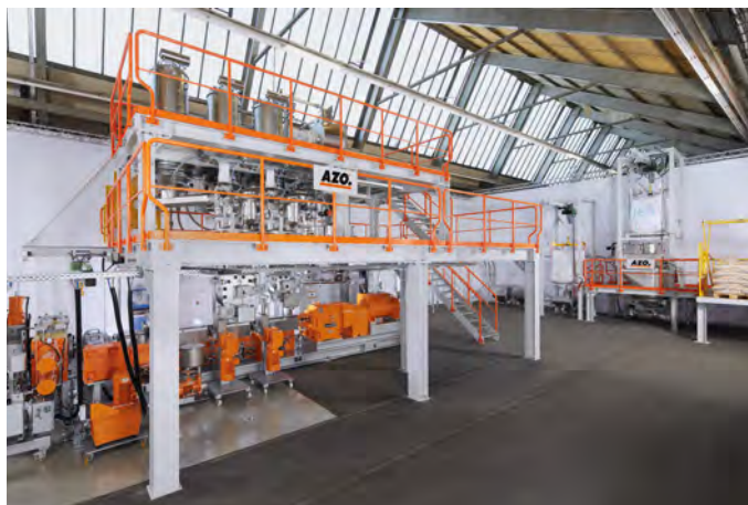
Feeding of raw materials, dosing and extruder for producing highly filled compounds
