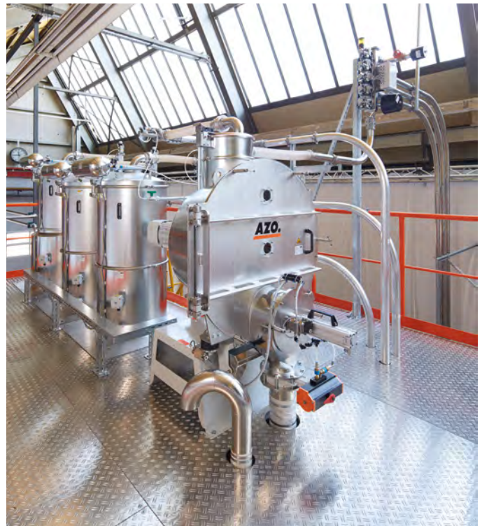
Receiver for feeding the AZODOS® units and AZO® MIXOMAT for producing premixes
