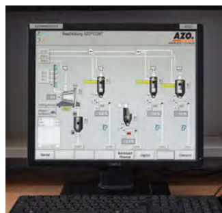
Visualisation of feeding of dosing units
