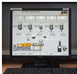
Visualisation of AZODOS® units and extruder
