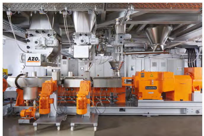
AZODOS® units for continuous gravimetric extruder filling
