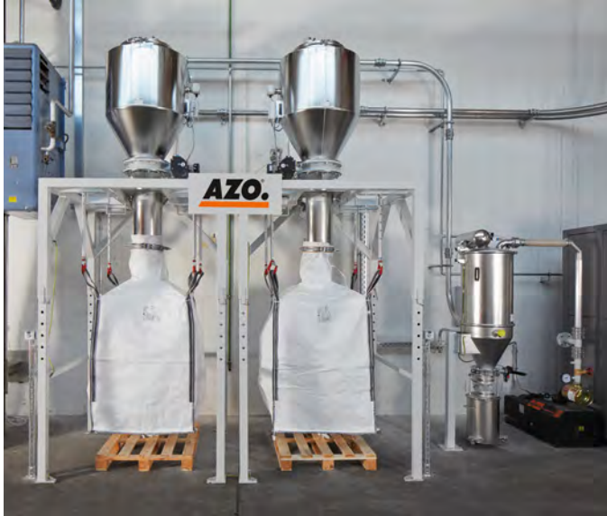
Filling of finished goods into big bags using a vacuum conveying line
