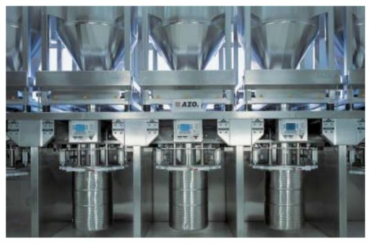
Centralized weighing of active and carrier ingredients into drums via the DOSITAINER®.
