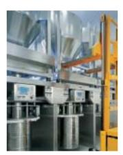
The BATCHTAINER® is taken to the individual filling stations by means of a fork-lift truck.
