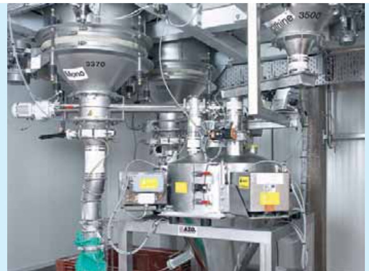
Automatic weighing of baking ingredients accurate to the gram
