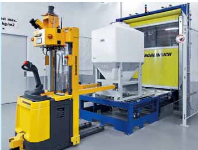
Storage and removal of DosiBoxes® with automated guided vehicles
