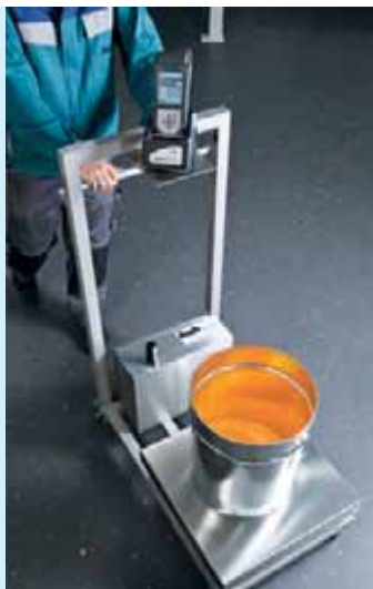
ManDos mobile: Highly flexible due to movable scale and mobile terminal with WLAN connection
