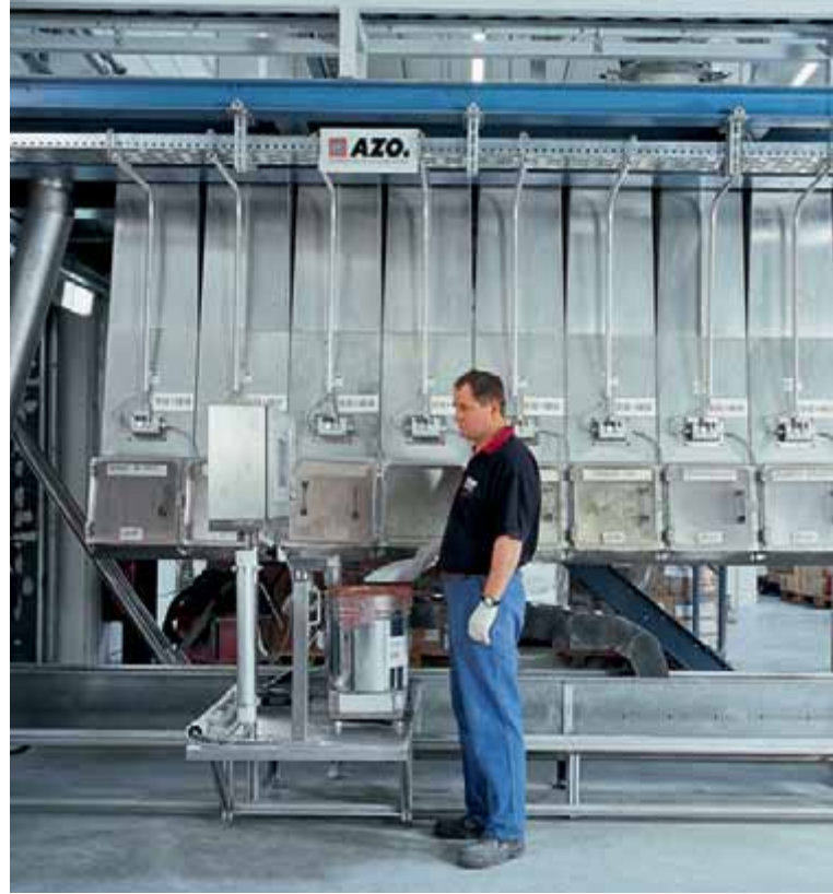
Operator-guided weighing of colours and additives
