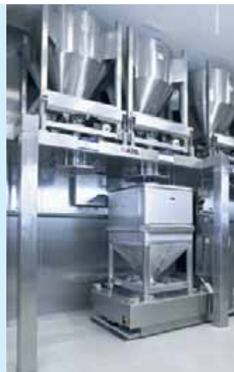
Linear arrangement of AZO DOSITAINERS®
