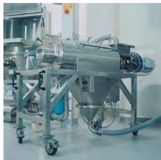
Screening in the conveying stream
