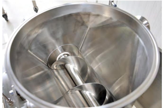
Inlet area free of dead space minimises product residue in dosing module
