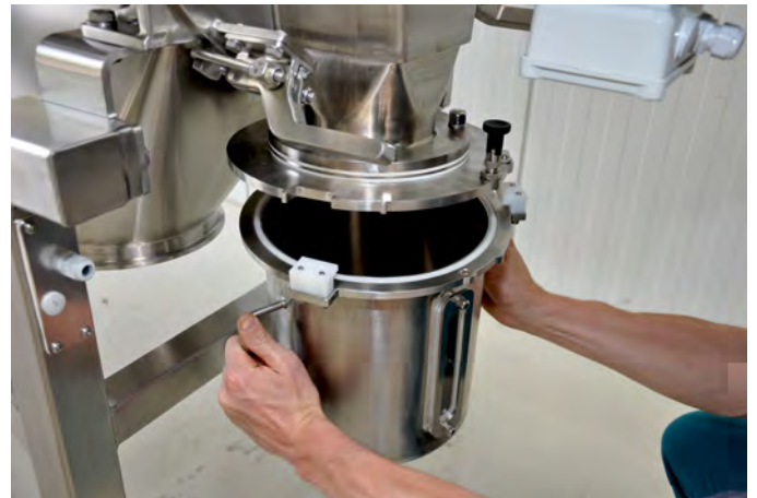
Coarse product collecting hopper with bayonet catch for easy removal without tools
