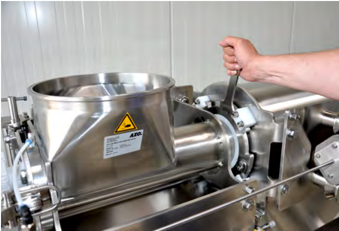
Various connection options between dosing and screening modules: bayonet catch, flange connection, welded
