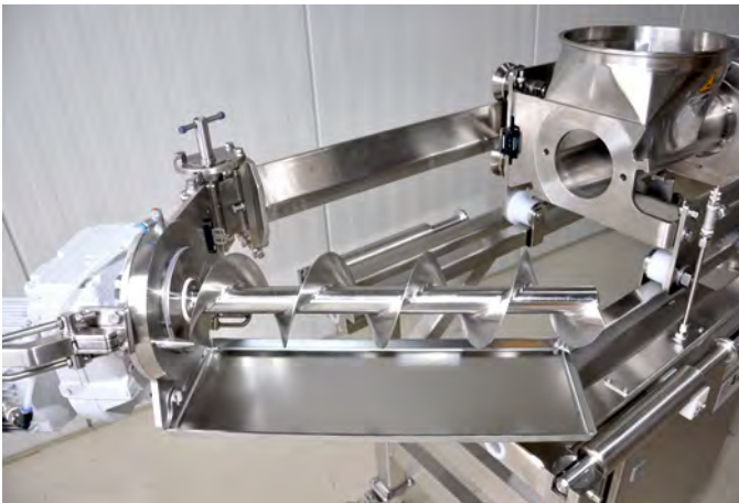
Trickle guard prevents soiling when removing the dosing screw
