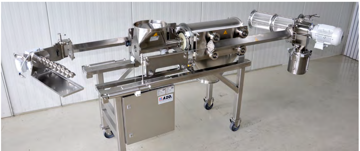
The screen and infeed can be extracted and swivelled to the side for quick inspection and cleaning
