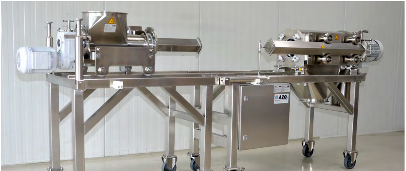
Adapter frame for easy installation of replaceable dosing modules
