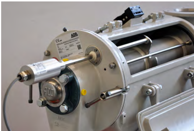
Screen basket with ultrasonic converter. The frequencies were transmitted to the wire mesh via the middle screen ring. The stainless steel wire mesh is bonded with the screen rings.
