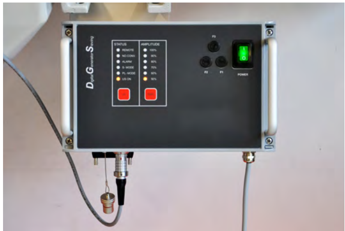
Generator for the generation of ultrasonic frequencies inclusive controls
