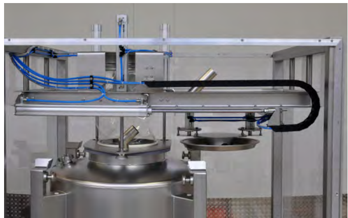
Dust-tight connection has been created, weighing of product into container is starting
