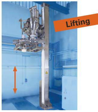
Up to 6 different positions can be assumed for the various working steps, e.g. loading at floor level, several working positions, servicing.
