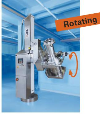
With the new Lifting column it is possible to rotate packing drums and empty them after docking with hoppers or processing equipment.
