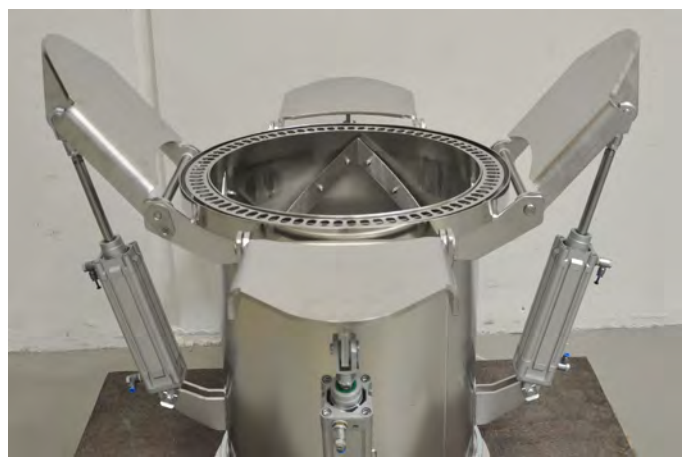
Massager device to help discharge
