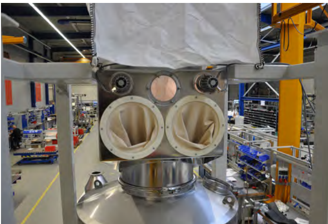
Big bag vacuum docking system with gloves
