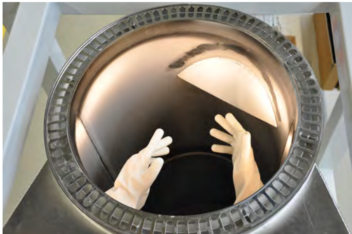
Circular vacuum aspiration for dust-free docking and fixing the big bag in place Alternative: with gloves
