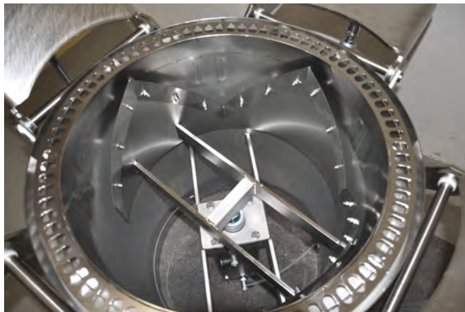
Circular vacuum aspiration for dust-free docking and fixing the big bag in place Alternative: with slitting device
